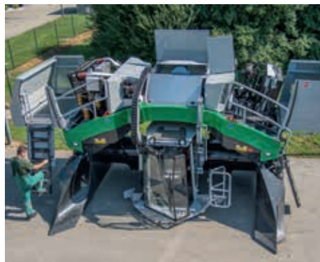
The hydraulically extendable maintenance platforms make for fast and easy maintenance.
