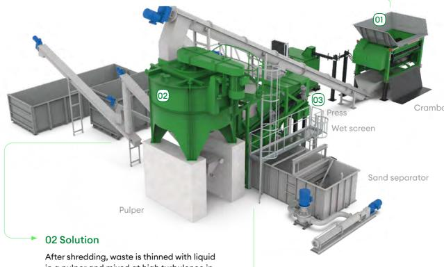
After shredding, waste is thinned with liquid in a pulper and mixed at high turbulence in batches. Items that are still packaged are thus separated into content and packaging material. After processing for a period depending on the material, the pulper is emptied. The liquid goes to wet screening, while heavy materials like metal, glass, bone, stones and ceramics are ejected discontinuously by a heavy materials separator.
