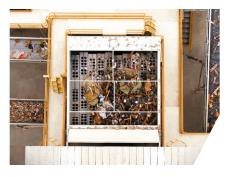
This electric-drive waste separator screens and separates 2D, 3D, and fines fractions in a single process, maximizing material sorting and recovery downstream.
